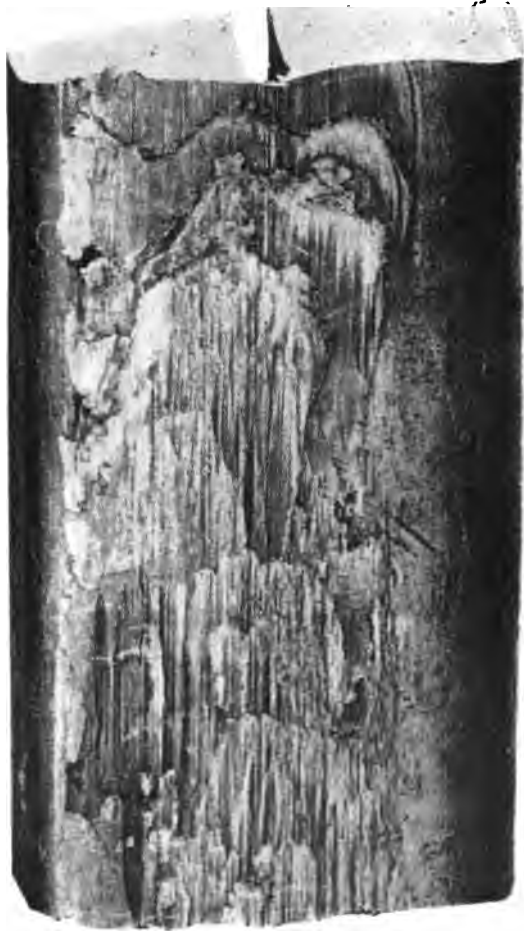
PHOTOGRAPH OF RUNNING SURFACE OF HEAD OF STEEL RAIL.
